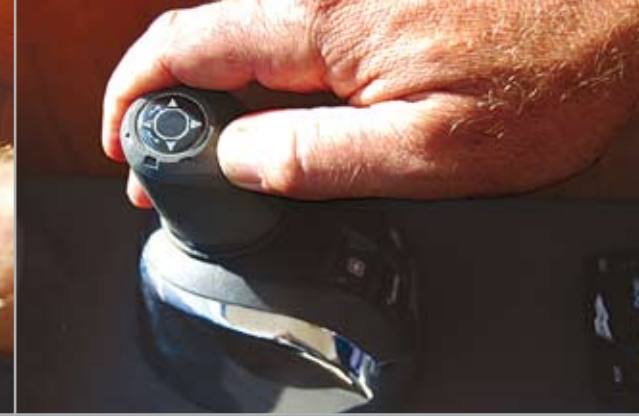
Push the joystick towards the port bow for forward sideways control
