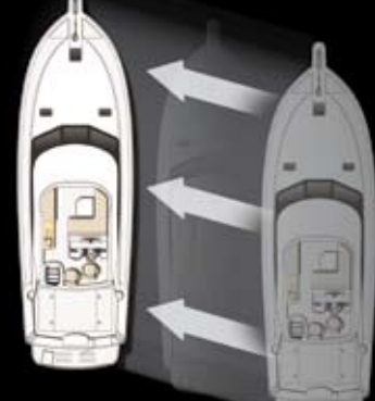
Push the joystick towards the port bow for forward sideways control
