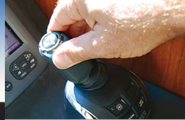
Push the joystick to port for sideways control
