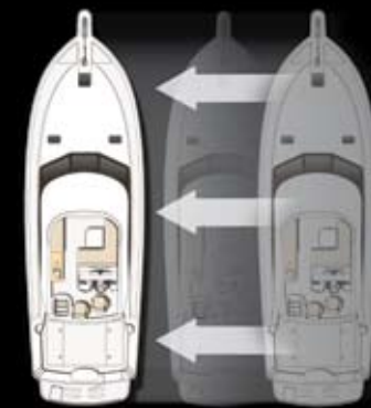
Push the joystick to port for sideways control
