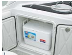
Cockpit wetbar with sink, faucet, S/Steel handrail and cooler storage with doors.
