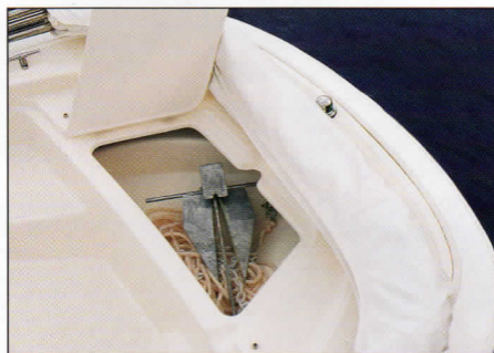
The bow locker with fiberglass cover and drain conceals the anchor and rode.
