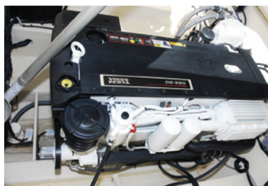
Engine Compartment with Full 360° Access VOLVO PENTA D-6 370 Turbo Diesel
