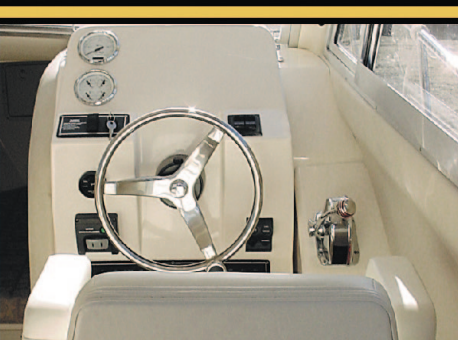
Helm station features plenty of room for electronics, single lever shift & throttle controls.
