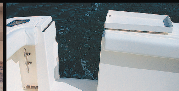
Large door swings out and features heavy duty stainless steel hinges and flip up lid.
