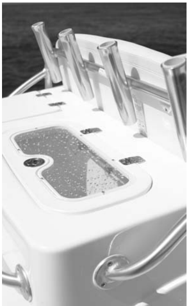
THE 50-GALLON LIGHTED LIVEWELL features a see-through lid so anglers can constantly monitor the health of their bait supply.
