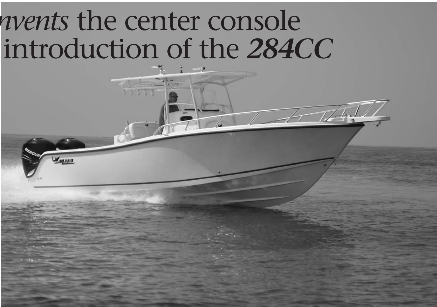
A SMOOTH RIDE is made possible by a foam-injected hull with full-length fiberglass stringers, trim tabs and a 21-degree deadrise.
