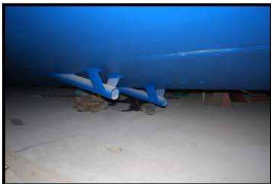
Port and centre shaft logs
