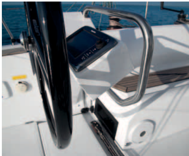
Rotating plotter pods on pedestals with stainless steel grab rails for control and safety.
