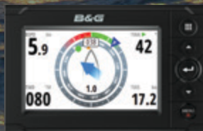
2 B&G H5000 multifunction displays, one at each helm position, B&G Autopilot, 2 H5000 control units & fluxgate Gyro Compass RC42, AIS Class B transponder, GoFree wireless link, Antenna for VHF, FM and AIS, incl. splitter
