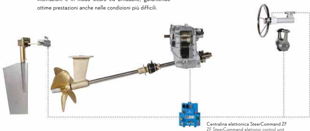
Sistema Steering by Wire sviluppato da Ferretti in collaborazione con ZF Steering by Wire system jointly developed by Ferretti and ZF
