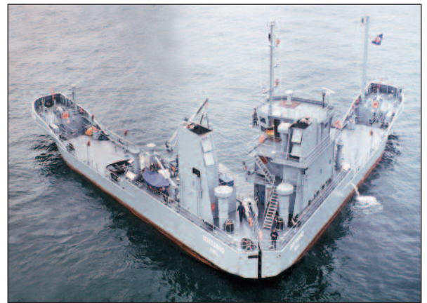
Pollution control and recovery vessel 2 x SRP 350 LS CP (600 kW each) Shipyard: C. Lühring, Germany Owner: German Navy
