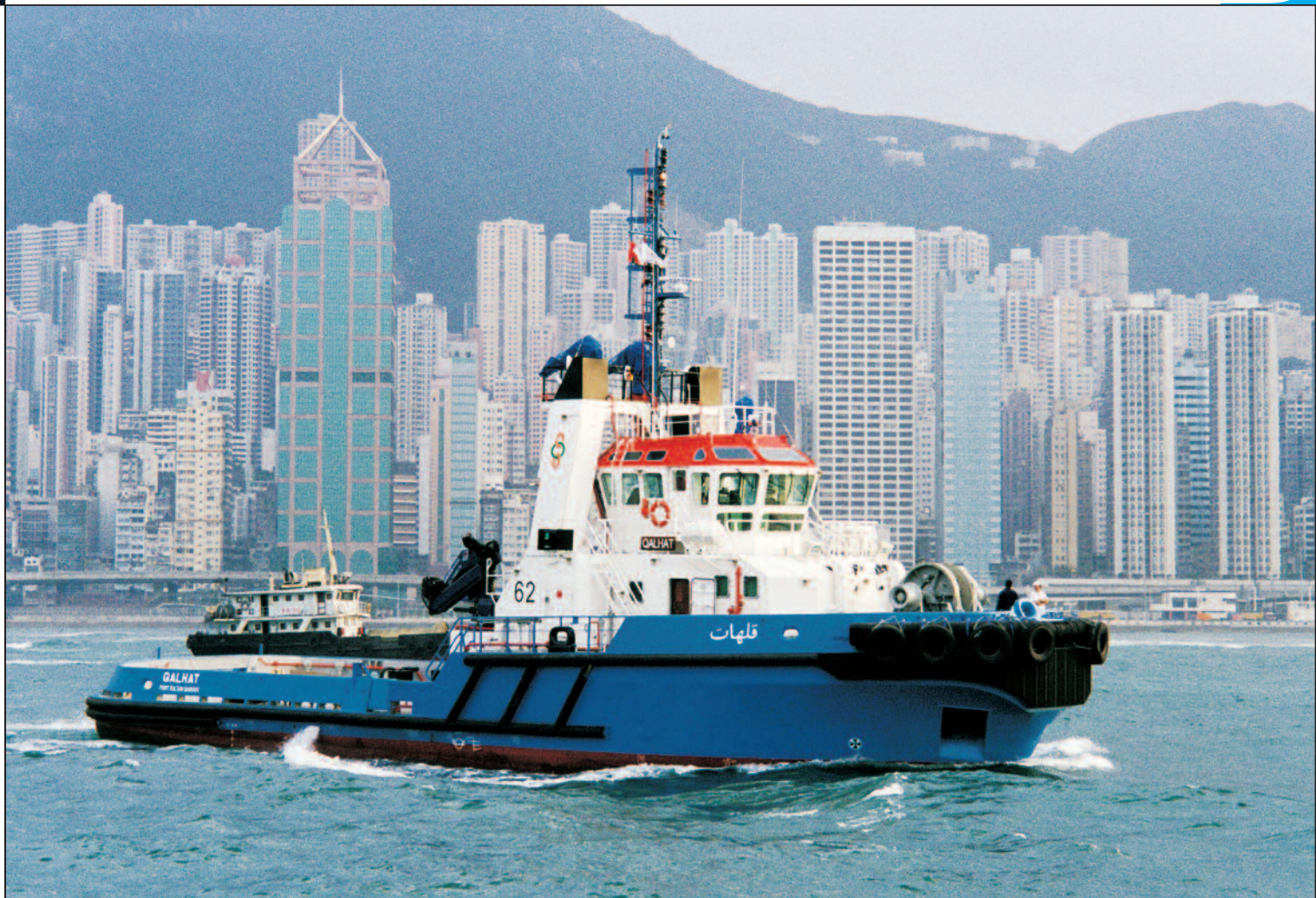
Stern tug, 2 x SRP 1515 CP (1850 kW each), 60 t bollard pull Shipyard: Cheoy Lee Shipyards Ltd, Hong Kong Owner: Wijsmuller Salvage BV, The Netherlands
