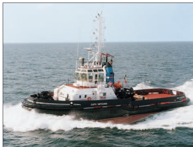
Stern tug, 2 x SRP 1212 CP (1545 kW each), 50 t bollard pull Shipyard: Damen Shipyards, The Netherlands Owner: Rimorchiatori Spezzini, Italy
