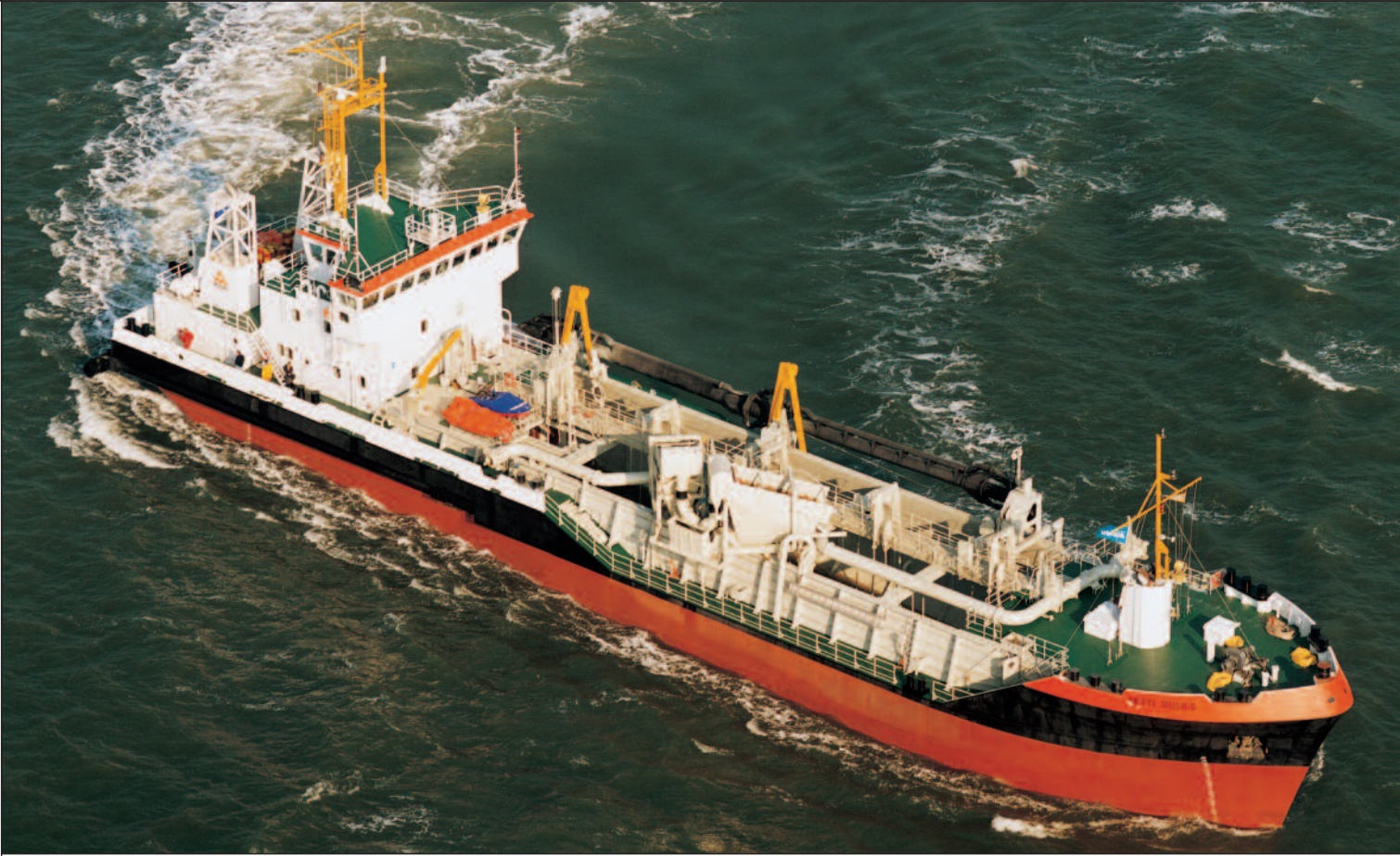
Suction hopper dredger, 2 x NAV 1010 (876 kW each) Shipyard: Scheepswerf Bijholt, The Netherlands Owner: Naßbaggerei Anton Müsing, Germany
