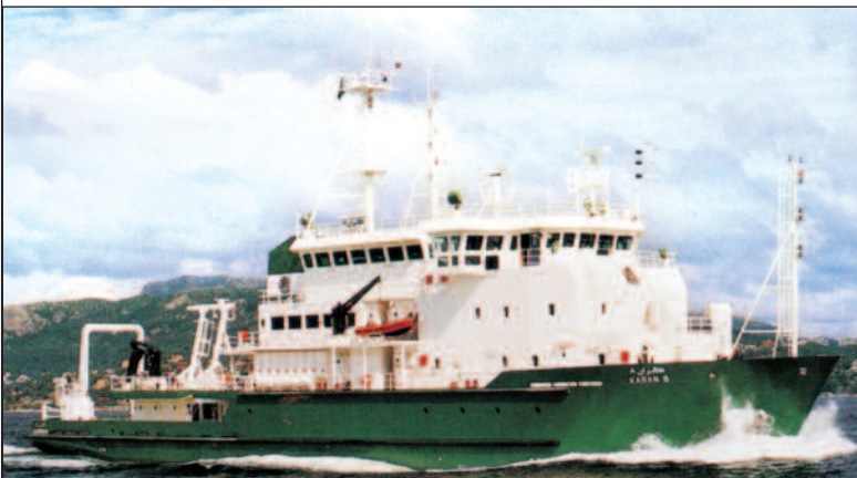
Research vessel 2 x SRP 1010 (900 kW each) Shipyard: Mjøllem & Karlsen, Norway Owner: ARAMCO, Saudi Arabia
