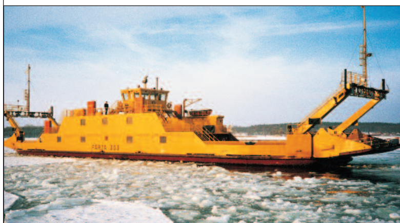
Double-ended ferry, 2 x SRP 350/350 (404 kW each) Shipyard: Åsi Verken, Sweden Owner: Swedish National Road Administration and Ferry Operation, Sweden
