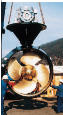
Tractor tug, 2 x SRP 1010 (1325 kW each), 45 t bollard pull Shipyard: Astilleros Zamakona, Spain Owner: Remolcadores de Barcelona, Spain
