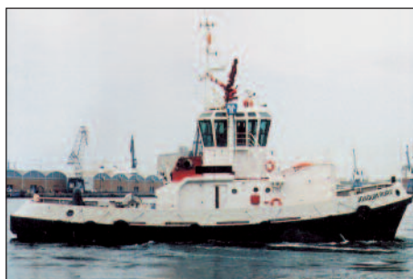
Tractor tug, 2 x SRP 1010 (1325 kW each), 45 t bollard pull Shipyard: Astilleros Zamakona, Spain Owner: Remolcadores de Barcelona, Spain
