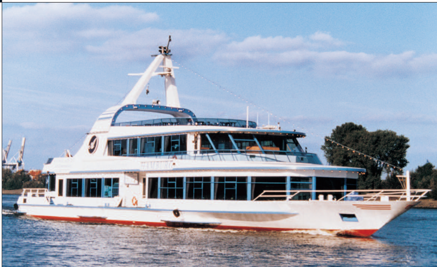
Passenger vessel, 2 x SRP 170 (284 kW each) Shipyard: Deutsche Binnenwerften GmbH, Germany Owner: Rainer Abicht Elbreederei GmbH, Germany
