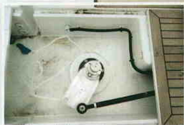
ABOVE Lewmar's flush-fitting hatches were designed into the coachroof, where lines run aft from the mast in troughs. Some more non-slip would be a useful addition. Note the plinth for the self-tacking jib track. LEFT To reach the steering linkage you simply lift a section of the cockpit sole
