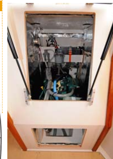
Campionway lifts on gas struts for engine access.
